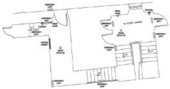
ACCESS STAIR PLAN (1:50) (GROUND TO 1st FLOOR)
